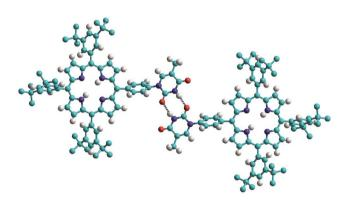
Fig. 2 View of the single crystal X-ray structure of mono-TP illustrating the formation of the inter-thymine  $R_2^2(8)$  double hydrogen-bonding interaction (represented with the two dotted lines) observed in the solid state. Hydrogen atoms of the *tert*-butyl groups are omitted for clarity. Atoms are colored as follows C – light blue; N – dark blue; H – white; O – red.
