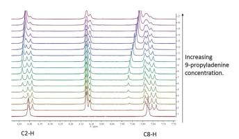
Fig. 3 <sup>1</sup>H NMR spectrum illustrating shifts in the C8–H and C2–H proton signals during titration of mono-TP with 9-propyladenine. Spectrum 1 corresponds to pure 9-propyladenine and spectra 2–17 are recorded with constant mono-TP concentration and increasing 9-propyladenine concentration.
