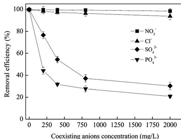
Fig. 9 Effect of coexisting anions on adsorption of Cr(vi) on CoFe<sub>2</sub>O<sub>4</sub>/MgAl-LDH.
