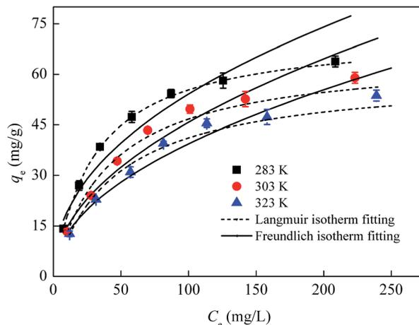
Fig. 5 Adsorption isotherm of Cr(vi) on CoFe<sub>2</sub>O<sub>4</sub>/MgAl-LDH at temperatures of 283, 303, 323 K.
