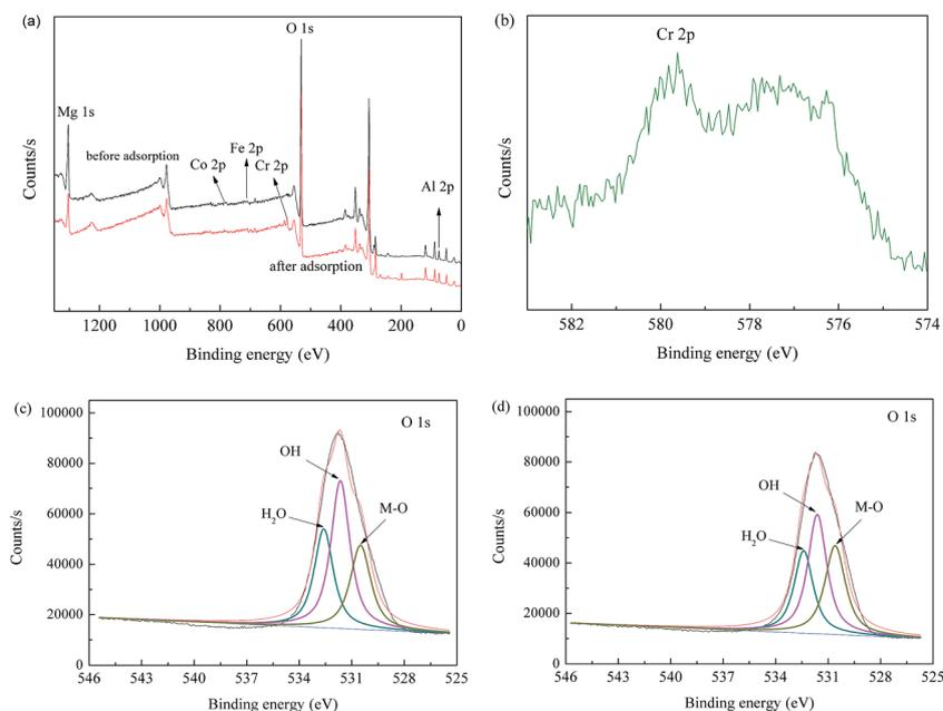
Fig. 7 Wide XPS spectra of (a) CoFe<sub>2</sub>O<sub>4</sub>/MgAl-LDH before and after Cr(vi) adsorption, (b) Cr 2p spectrum of CoFe<sub>2</sub>O<sub>4</sub>/MgAl-LDH after Cr(vi) adsorption, (c) O 1s spectrum of CoFe<sub>2</sub>O<sub>4</sub>/MgAl-LDH, and (d) O 1s spectrum of CoFe<sub>2</sub>O<sub>4</sub>/MgAl-LDH after Cr(vi) adsorption.
