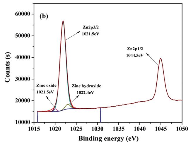
Fig. 2 XPS spectra of (a) biochar before and after modification; (b) zinc  $2p_{3/2}$  of zinc–biochar.
