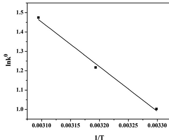
**Fig. 11** Plot of  $\ln k^0$  versus  $1/T$  for estimation of thermodynamic parameters for the adsorption of Cr(vi) on zinc-biochar (volume: 50 mL; adsorbent dose: 0.1 g; initial Cr(vi) concentration: 25, 50, 75, 100, 200, 250, 400, 500 mg L<sup>-1</sup>; pH: 2.0; contact time: 24 h).
