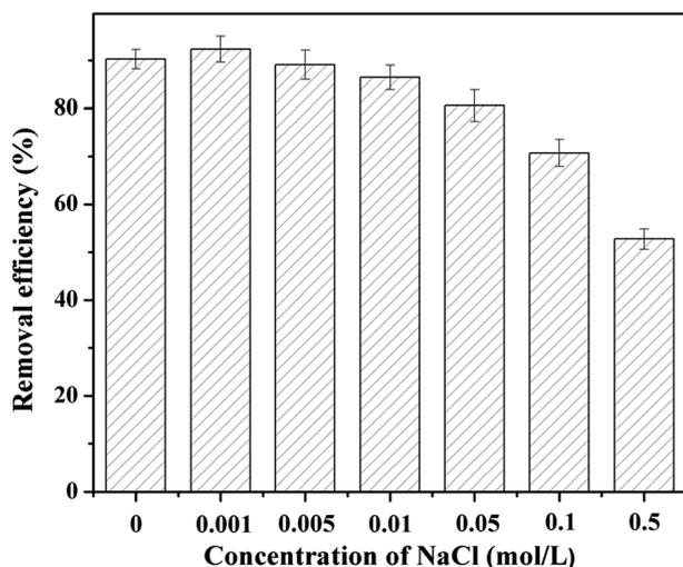
Fig. 12 Effect of different concentrations of NaCl on Cr(vi) removal by zinc-biochar (volume: 50 mL; adsorbent dose: 0.1 g; initial Cr(vi) concentration: 50 mg L<sup>-1</sup>; pH: 2.0; contact time: 24 h).
