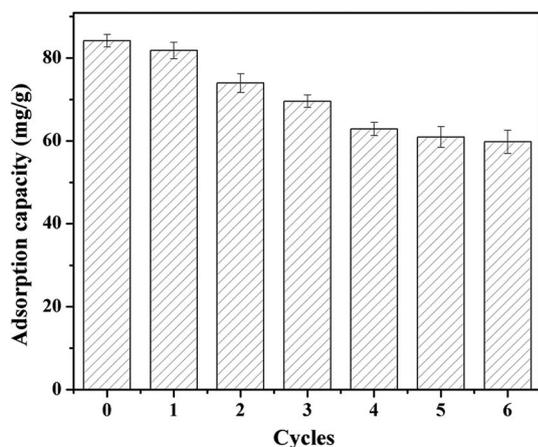
Fig. 13 Sixth consecutive adsorption-desorption cycles of zinc-biochar for Cr(vi) removal (volume: 50 mL; adsorbent dose: 0.1 g; initial Cr(vi) concentration: 500 mg L<sup>-1</sup>; pH: 2.0; contact time: 24 h).
