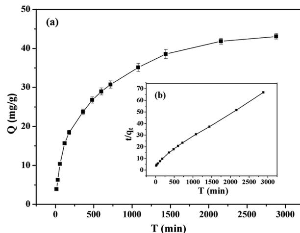
Fig. 9 Kinetics of Cr(vi) adsorption onto the zinc-biochar at 303.15 K (initial Cr(vi) concentration  $100 \text{ mg L}^{-1}$ ; pH: 2.0). (a) Cr(vi) sorption kinetics data; (b) pseudo-second-order model for Cr(vi) adsorption.
