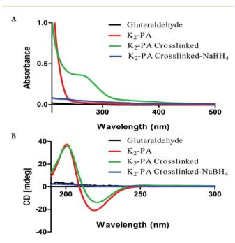
Fig. 2 UV-Vis spectroscopy (A) and circular dichroism (B) analysis of peptide gels and crosslinked peptide gels at pH 7.5.
