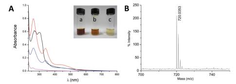
Fig. 2 (a) UV-Vis spectra of aqueous solutions of 1 (black) and  $1/C_{60}$  nanocomposites obtained by HSVM (red), manual grinding (blue) and sonication (pink). Inset: picture of the solutions obtained by HSVM (a), manual grinding (b) and sonication (c). (b) MALDI-TOF mass spectrum of the solution obtained by HSVM.
