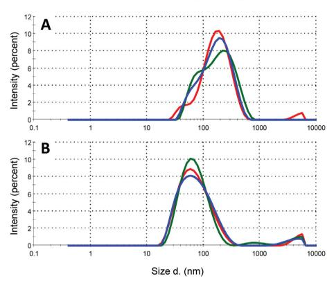
Fig. 5 DLS of the aqueous solutions of 1/C<sub>60</sub> nanocomposites obtained by HSVM: (a) upon centrifugation at 4000 rpm, (b) upon centrifugation at 14 000 rpm.
