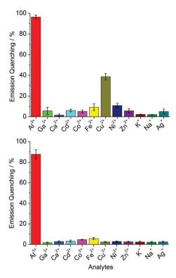
Fig. 2 Top: fluorescence emission quenching ( $\lambda_{ex}=490$  nm;  $\lambda_{em}=505$  nm) of buffered aqueous solutions (10 mM MOPS, pH 7.0, H<sub>2</sub>O with 0.6 vol% MeOH) of dye 4 (4.0  $\mu$ M) in the presence different metal cations (60  $\mu$ M). Bottom: measurements in the presence of the masking agent histidine (5.0 mM). The values are averages of three independent measurements.
