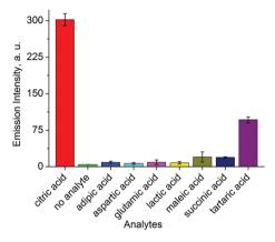
Fig. 5 Fluorescence emission intensity ( $\lambda_{ex}$  = 490 nm;  $\lambda_{em}$  = 505 nm) of buffered aqueous solutions (10 mM MOPS, pH 7.0, H<sub>2</sub>O with 1.2 vol% MeOH) of dye 4 (4.0  $\mu$ M) and Al<sup>3+</sup> (120  $\mu$ M) in the presence different analytes (400 µM). The values are averages of three independent measurements.
