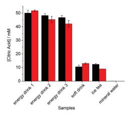
Fig. 6 Concentration of citric acid in drinks as determined by  $^1H$  NMR spectroscopy (black bars) and by the dye  $4-Al^{3+}$  sensing ensemble (red bars). Experimental details are given in the ESI.†
