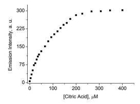
Fig. 4 Fluorescence emission intensity ( $\lambda_{ex}$  = 490 nm;  $\lambda_{em}$  = 505 nm) of buffered aqueous solutions (10 mM MOPS, pH 7.0, H<sub>2</sub>O with 1.2 vol% MeOH) containing dye 4 (4.0 μM), Al<sup>3+</sup> (120 μM), and different amounts of citric acid (0-400  $\mu$ M). The data points are averages of three independent measurements. The errors are less than 4%.
