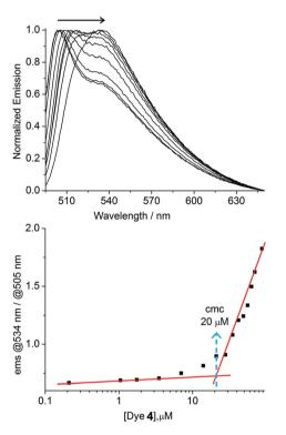
Fig. 1 Top: normalized fluorescence emission spectra ( $\lambda_{ex}$  = 490 nm) of buffered aqueous solutions (10 mM MOPS, pH 7.0) containing different amounts of dye 4 (0.21–105  $\mu$ M). Bottom: relative fluorescence intensity at 534 and 505 nm of the same solutions.
