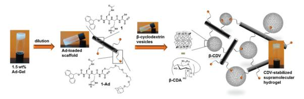
Fig. 9 Formation of a stabilized supramolecular hydrogel of adamantane functionalized peptide scaffolds (1:1-Ad mixed 9:1 and cyclodextrin vesicles (CDV) of amphiphilic β-cyclodextrin host molecules (β-CDA) via multivalent host-guest inclusion complexes at pH 6 (final concentrations are 0.75 wt% of 1 and 2 mM (0.6 wt%) CDV).
