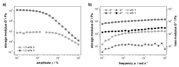
Fig. 2 Oscillatory rheological measurements of solutions and hydrogels with 1.0 wt% and 1.5 wt% 1. (a) Storage modulus obtained from a strain-amplitude sweep performed at  $\omega = 10$  rad s<sup>-1</sup>. (b) Storage G' and loss G'' moduli obtained from a frequency sweep performed at  $\gamma = 0.5\%$ .
