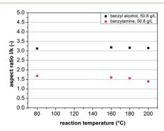
Fig. 10 Influence of the reaction temperature on the aspect ratio of the AZO nanocrystals prepared in BnOH and BnNH<sub>2</sub>.
