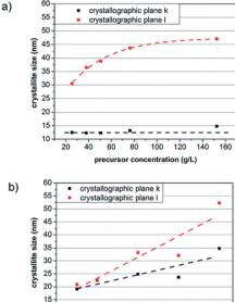
Fig. 5 Crystallite size as a function of the precursor concentration of a) the AZO nanorods synthesized in benzyl alcohol and b) the AZO nanocrystals prepared in benzylamine.
