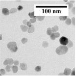
Fig. 2 TEM images of the rod-shaped AZO nanoparticles obtained in BnOH at a precursor concentration of 50.8 g L<sup>-1</sup> (left) and the spherical AZO nanoparticles prepared in BnNH2 at a precursor concentration of 25.4 g L<sup>-1</sup> (right).
