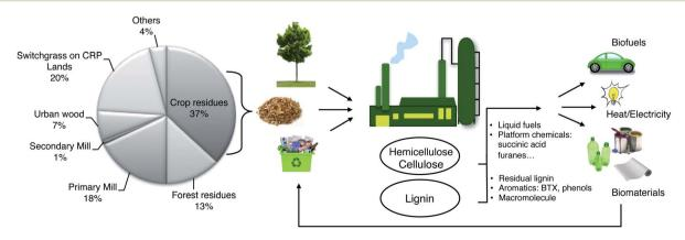
Fig. 2 Cartoon showing the role of the future biorefinery as part of a fully integrated agro-biofuel-biomaterial-biopower cycle. The pie chart shows the distribution of vegetal biomass by volume. (CRP = Conservation Reserve Program).
