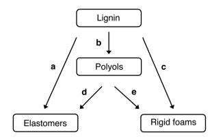
**Fig. 6** Synthetic routes for lignin incorporation in polyurethane materials: (a) direct use, (b) synthesis of liquid polyol, (c) synthesis of rigid polyurethane foams using lignin-based polyols, (e) synthesis of polyurethane elastomers using lignin-based polyols and (d) synthesis of rigid polyurethane foams using lignin as reactive filler. 98
