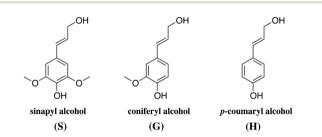
Fig. 3 The three main monomer building blocks of lignin.
