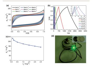
Fig. 5 Electrochemical performance of BD-700-A3 based on the two-electrode system: (a) CVs at different scan rates; (b) galvanostatic charge/discharge curves and (c)  $C_{\rm s}$  at various current densities; (d) coin cell stacks made of BD-700-A3 light up a LED. The current densities were calculated based on the mass of active materials on one electrode.
