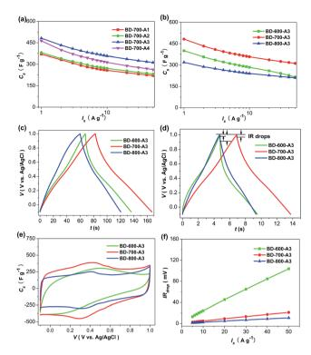
Fig. 6 Electrochemical performance comparisons of carbon materials activated at various conditions based on the three-electrode system: (a and b)  $C_s$  at various current densities; galvanostatic charge/discharge curves collected at (c) 5 A g $^{-1}$  and (d) 50 A g $^{-1}$ ; (e) CVs at 200 mV s $^{-1}$ ; (f) IR<sub>drops</sub> collected at various current densities.
