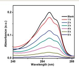
Fig. 11 UV-vis spectrum of decomposition of phenol using ZnO/Au catalyst, under irradiation of visible light. Conditions: [phenol] =  $2 \times 10^{-4}$  M and amount of catalyst = 50 mg.
