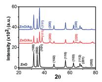
Fig. 3 Powder X-ray diffraction (PXRD) patterns of ZnO, ZnO/Au, and ZnO/Ag nanoparticles. During scan  $2\theta$  values varies from  $20-80^\circ$  and the scanning rate was fixed at  $2^\circ$  per min.
