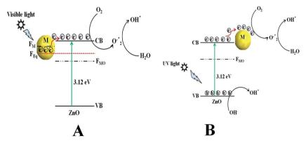
Scheme 2 The overall dye degradation mechanism under irradiation of (a) visible light and (b) UV light, with ZnO/Au and ZnO/Ag nanoparticles. Here, VB = valence band, CB = conduction band,  $F_{MO} = Fermi level of metal oxide$ ,  $F_{M} = Fermi level of metal$ ,  $F_{Eq} = Fermi level of equilibrium$ , and M = Au and Ag.
