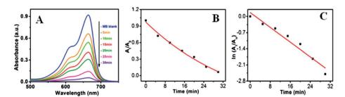
Fig. 10 UV-vis spectra of (a) degradation of MB dye in presence of ZnO/Au under visible light (b)  $A_t/A_0$  vs. time (min) plot and (c)  $\ln A_t/A_0$  vs. time (min) plot. During the photocatalysis measurements, reaction mixture was stirred continuously. Conditions: [MB] =  $10^{-5}$  M and amount of catalyst = 50 mg.
