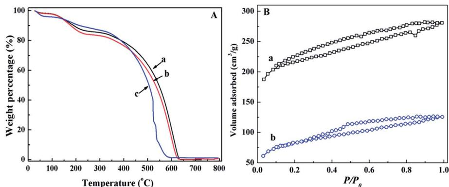
Fig. 7 (A) TGA curves of PANI/CF (a) before and after treating with (b) 8.0 and (c) 32.0 mg L<sup>-1</sup> Cr(vi) solution; (B) the nitrogen adsorption-desorption isotherm of PANI/CFs with a 10.0 wt% loading after treated with (a) 4.0 and (b) 12.0 mg L<sup>-1</sup>.
