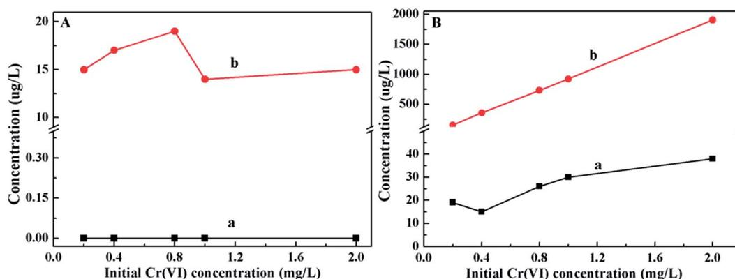
Fig. 6 Cr(vi) (a) and total Cr (b) concentrations in the solution (A) and PANI/CFs (B) after adsorption with initial Cr(vi) concentrations ranging from 0.2 to 2.0 mg L<sup>-1</sup>.
