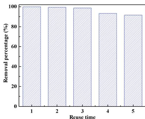
Fig. 8 Cr(vi) removal efficiency of the regenerated PANI/CFs after 60 min adsorption. ([Cr(vi)]: 4.0 mg L<sup>-1</sup>, [PANI/CF]: 55.0 mg, pH: 1.0, treating time: 60 min).
