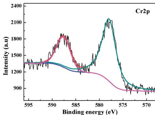
**Fig. 5** XPS Cr2p spectra on PANI/CFs after the adsorption of Cr(vi) solution with an initial concentration of 48.0 mg L<sup>-1</sup> and pH of 1.0.
