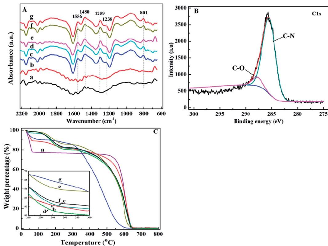
Fig. 2 (A) FT-IR spectra of the (a) as-received CFs, (b) CFs washed by HNO<sub>3</sub>, PANI/CFs with a PANI loading of (c) 5.0, (d) 10.0, (e) 15.0, (f) 20.0 wt%, and (g) pure PANI; (B) XPS C1s spectra of the synthesized PANI/CFs with a PANI loading of 10 wt%; and (C) TGA curves of (a) the as-received CFs, (b) CFs washed by HNO<sub>3</sub>, PANI/CFs with a PANI loading of (c) 5.0, (d) 10.0, (e) 15.0, (f) 20.0 wt%, and (g) pure PANI, respectively.
