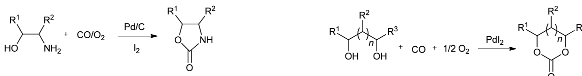
Scheme 11 Reagents and conditions: ethanolamine (10 mmol), Pd/C (0.01 mmol), promoter (0.036 mmol), temp. 100 °C, CO (1.0 MPa), O 2 (0.25 MPa), DME (8 mL), time 1 h.
