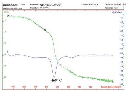
Fig. 4 TGA curves of NP-C[8]-C<sub>4</sub>-COOH.
