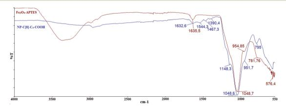
Fig. 2 FTIR spectra of Fe<sub>3</sub>O<sub>4</sub>-APTES and NP-C[8]-C<sub>4</sub>-COOH
