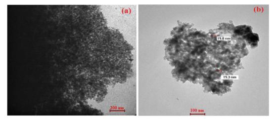
Fig. 3 TEM micrographs of (a) Fe<sub>3</sub>O<sub>4</sub>-nanoparticles and (b) NP-C[8]-C<sub>4</sub>-COOH.
