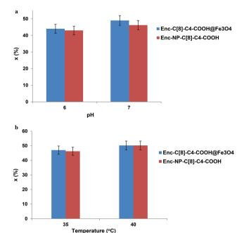
**Fig. 7** Effect of pH (a) and temperature (b) on the conversion (x) in the hydrolysis of racemic naproxen methyl ester. Averages and standard deviations calculated for data received from three independent extraction experiments.
