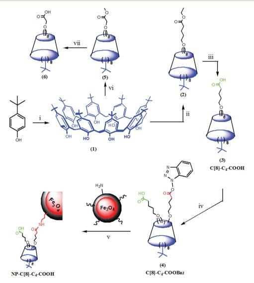
Scheme 1 Preparation of C[8]- $C_4$ -COOH and NP-C[8]- $C_4$ -COOH. Reaction conditions: (i) paraformaldehyde, NaOH; (ii)  $K_2CO_3$ , NaI, 5-bromovale-rate; (iii) 15% NaOH solution; (iv) 1-hydroxybenzotriazole, DCC; (v)  $Fe_3O_4$ -APTES; (vi) methylbromoacetate,  $K_2CO_3$ ; (vii) 15% NaOH solution.
