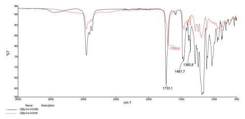
Fig. 1 FTIR spectra of C[8]-C<sub>4</sub>-COOEt and C[8]-C<sub>4</sub>-COOH.
