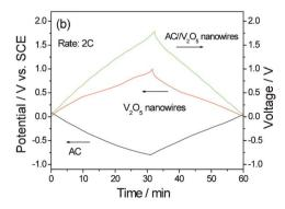
Fig. 12 (a) CV curve of  $V_2O_5$  nanowires and Ni mesh (current collector) and (b) charge/discharge curves of AC// $V_2O_5$  nanowires in 0.5 mol I<sup>-1</sup> K<sub>2</sub>SO<sub>4</sub> aqueous solution (modified from ref. 6a).
