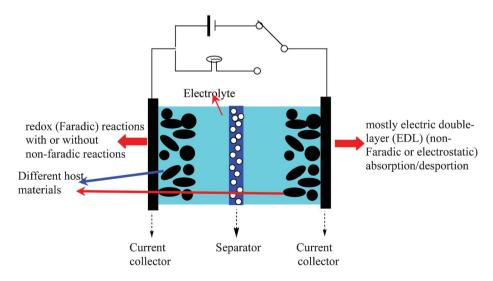
Fig. 1 Schematic illustration of ASCs.
