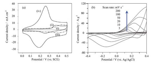
Fig. 14 (a) CV curves of various electrodes at 50 mV s<sup>-1</sup> in 1 mol l<sup>-1</sup> KOH solution; (i) CNTs: (ii), nickel oxide/CNTs; (iii) cobalt oxide/CNTs; (iv), nickel-cobalt oxides/ CNTs (Ni/Co molar ratio = 1 : 1), and (b) CV curves of  $\alpha$ -Co(OH)<sub>2</sub> composite electrode recorded in 1 mol l<sup>-1</sup> KOH aqueous solution at different scan rates (modified from ref 84a and 85c)
