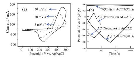
Fig. 15 (a) CV curve of Ni(OH)<sub>2</sub> in alkaline solution and (b) charge/discharge curves of the positive and negative electrodes in the AC//Ni(OH)<sub>2</sub> ASC and electric double layer capacitors of AC//AC at 1 mA cm<sup>-2</sup> in 10 mol l<sup>-1</sup> KOH aqueous solution (modified from ref. 87b and 90c).
