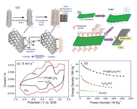
Fig. 3 Schematic illustration for the synthesis of (a)  $V_2O_5$ @CNTs (modified from ref. 37a) and (b)  $PPy@V_2O_5$ , (c) CV curves of  $V_2O_5$  and  $PPy@V_2O_5$  in 0.5 mol  $I^{-1}$   $K_2SO_4$ solution, and (d) Ragone plots of the ASC of  $V_2O_5$ //AC and  $PPy@V_2O_5$ //AC using 0.5 mol  $I^{-1}$   $K_2SO_4$  solution as the electrolyte (The capacitance and energy densities were calculated based on the total mass of two active electrode materials) (modified from ref. 6b).
