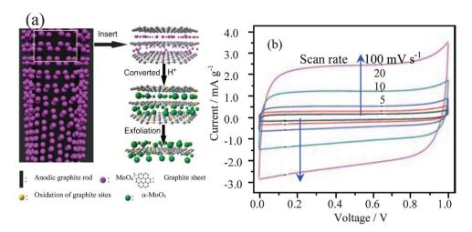
Fig. 11 (a) Illustration of the formation of the composite of  $\alpha$ -MoO<sub>3</sub>-decorated graphene sheets by electrolytic exfoliation from graphite with the assistance of molybdate and (b) CV curves of the composite in 6 mol l<sup>-1</sup> KOH (modified from ref. 49a).
