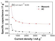
Fig. 6 (a) CV curves of an AC in 6 mol  $I^{-1}$  KOH aqueous electrolyte and (b) comparison of gravimetric capacitances against current density for the AC and the commercial Maxsorb carbon (modified from ref. 51b).
