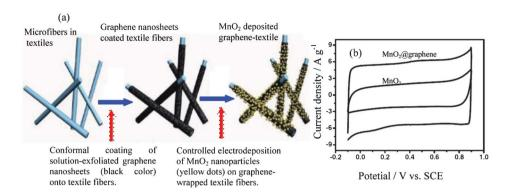
Fig. 9 (a) Schematic illustration of two key steps for preparing hybrid  $MnO_2$ -nanostructured textiles@graphene and (b) CV curves of an optimized  $MnO_2$ @graphene at different potential windows at the scan rate of 20 mV s<sup>-1</sup> in 1 mol l<sup>-1</sup>  $Na_2SO_4$  solution (modified from ref. 8a and 8b, respectively).
