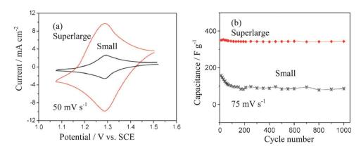
Fig. 13 (a) Typical CV curves and (b) cycling performance of super-large PbO<sub>2</sub> dendrites composed of trigonal nanoplates and the small dendrites in 5.0 mol  $I^{-1}$  H<sub>2</sub>SO<sub>4</sub> solution recorded a scan rate of 75 mV s<sup>-1</sup> (modified from ref. 82c).
