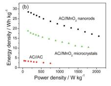
Fig. 10 (a) CV curve of MnO<sub>2</sub> in 0.5 mol I<sup>-1</sup> different neutral electrolytes and (b) Ragone plots of the hybrid supercapcitors AC//MnO<sub>2</sub> nanorods, AC//MnO<sub>2</sub> microcrystals supercapacitor and AC//AC supercapacitor in 0.5 mol I<sup>-1</sup> K<sub>2</sub>SO<sub>4</sub> electrolyte (modified from ref. 7c).
