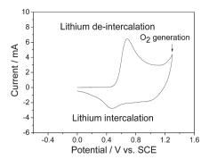
Fig. 18 CV curve of in LiNi<sub>1/3</sub>Co<sub>1/3</sub>Mn<sub>1/3</sub>O<sub>2</sub> in 2 mol  $I^{-1}$  Li<sub>2</sub>SO<sub>4</sub> aqueous solution (modified from ref. 108).
