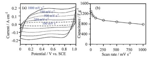
Fig. 8 (a) CV curves at different scan rates and (b) dependence of the capacitance on the scan rate for an annealed RuO<sub>2</sub>·xH<sub>2</sub>O nanotube arrayed electrode (0.19 mg cm $^{-2}$ ) in 1.0 mol I $^{-1}$  H<sub>2</sub>SO<sub>4</sub> solution (modified from ref. 54a).
