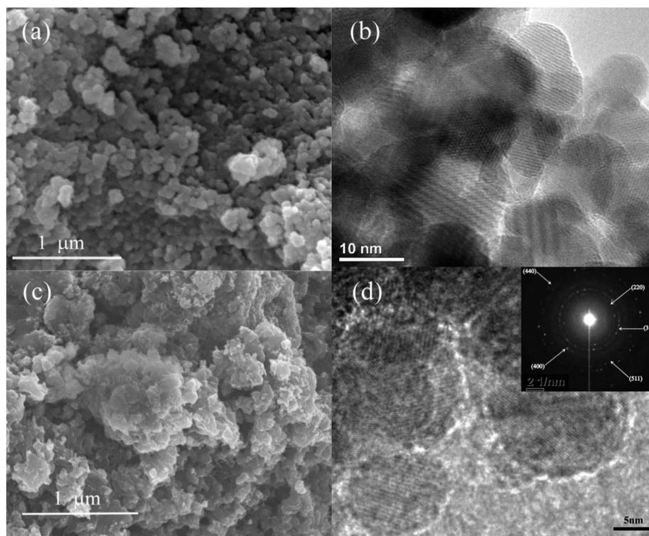
**Fig. 1** (a) SEM and (b) TEM images of the as-received  $\text{Fe}_3\text{O}_4$  NPs; (c) SEM image and (d) HRTEM image and selected area electron diffraction (SAED) pattern (inset picture) of the synthesized PNCs.
