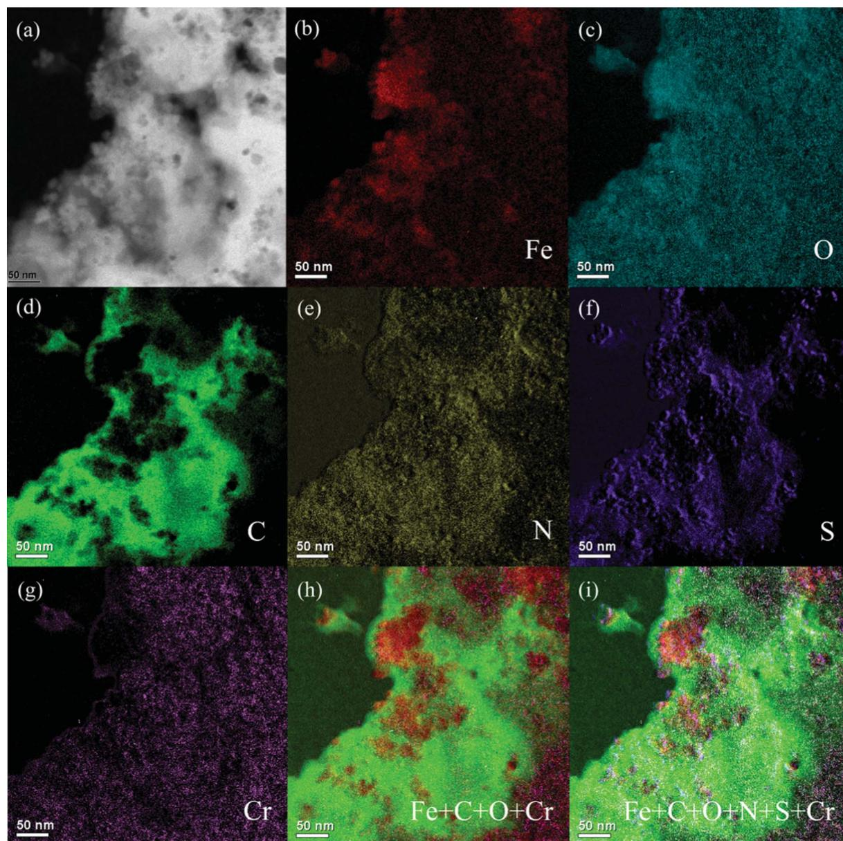
**Fig. 6** EFTEM of the PNCs after 5 min treatment with 20.0 mL Cr(VI) solution (pH = 1.0; 4.0 mg L<sup>-1</sup>): (a) zero-loss image, (b) Fe map, (c) O map, (d) C map, (e) N map, (f) S map, (g) Cr map, (h) Fe + C + O + Cr map, and (i) Fe + C + O + N + S + Cr map.
