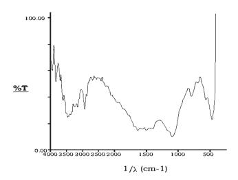
Fig. 2 Infra-red spectrum of activated bottom ash.
