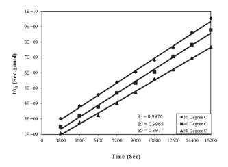
**Fig. 6** Plot of time *versus tlq<sub>t</sub>* for the Rose Bengal (pH = 7.2, concentration =  $5 \times 10^{-5}$  M)–bottom ash (0.50 g and mesh size = 100 BSS) system at different temperatures.
