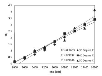
**Fig. 7** Time *versus B*<sub>t</sub> plot for Rose Bengal (pH = 7.2, concentration =  $5 \times 10^{-5}$  M)-bottom ash (0.50 g, mesh size = 100 BSS) adsorption at different temperatures.
