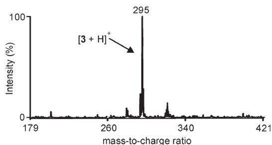
**Fig. 4** MALDI-TOF mass spectrum of the imine **3** ( $m/z = 295$ ) formed on-chip within the ionization chamber of the MALDI instrument and detected by extracting ions from the reaction mixture through the monitoring window.
