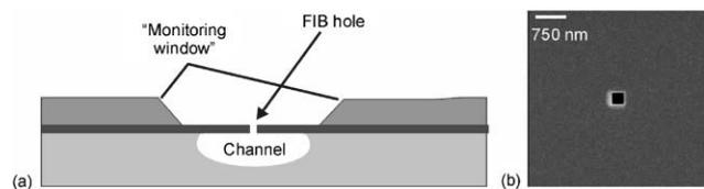
**Fig. 2** (a) Cross-section of the silicon-glass hybrid chip with a KOH etched “monitoring window” and a sampling hole above the HF microchannel. (b) SEM image of  $250 \times 250$  nm sampling holes made by FIB in the doped silicon layer.
