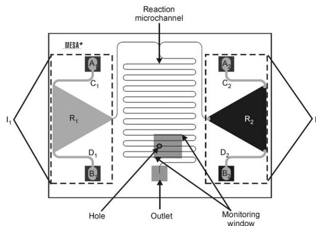
Fig. 1 Outline of the chip used to prove the “monitoring window” principle. Each inlet loading system ( $I_x$ ) consists of two inlet holes ( $A_x$  and  $B_x$ ) connected to a reservoir ( $R_x$ ) through channels  $C_x$  and  $D_x$  (with  $x = 1$  and  $2$ ).
