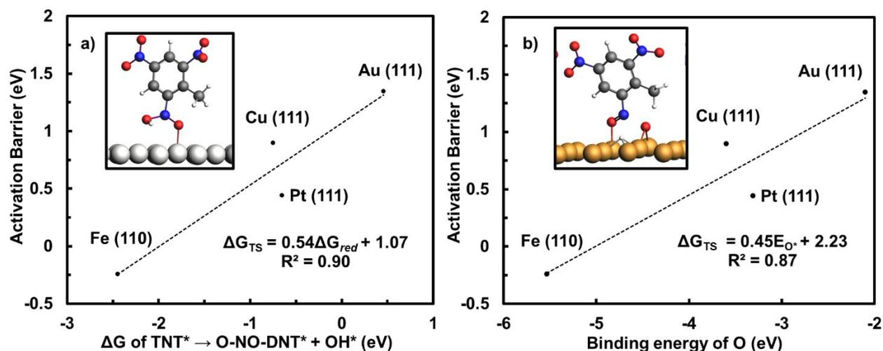
**Figure 7.** Brønsted–Evans–Polanyi relationship of a) initial reduction of TNT plots the activation barriers ( $\Delta G_{TS}$ ) versus the reaction energy ( $\Delta G_{red}$ ) for the reduction of TNT\* to O-NO-DNT + OH\* at 0 V-RHE on the Fe (110), Cu (111), Pt (111), and Au (111) metal surfaces. b) Correlation of the activation barriers for the reduction of TNT\* to O-NO-DNT\* + OH\* with the binding energy
