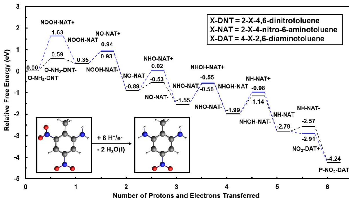
**Figure 2.** Reaction energy diagram for outer-sphere electrochemical reduction of O-NH<sub>2</sub>-DNT to P-NO<sub>2</sub>-DAT in the solution phase, calculated using the G16 code and IEFPCM solvation model. Reduction proceeds by reducing the second ortho  $\text{NO}_2$  group to the methyl group of TNT. Energies
