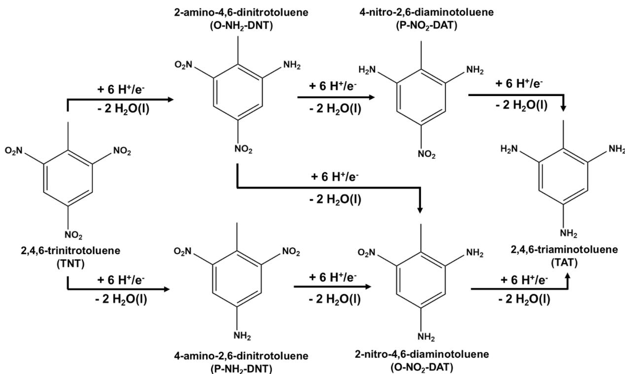
**Scheme 1:** Overall reaction for the electrochemical reduction of 2,4,6-tri-nitro-toluene (TNT) to 2,4,6-tri-amino-toluene (TAT).
