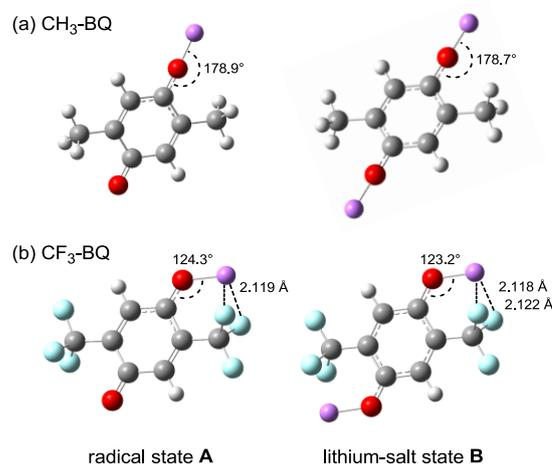
**Fig. 6** Optimized structures of (a) CH<sub>3</sub>-BQ and (b) CF<sub>3</sub>-BQ in radical **A** and dilithium-salt **B** states by DFT calculations. Atom colors : C, gray; H, white; O, red; F, aqua; Li, purple.
