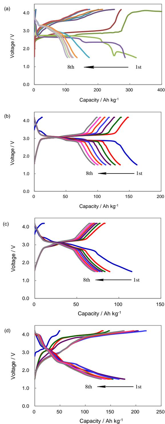
**Fig. 3** Charge-discharge curves and cycle-life performance over eight cycles for (a) CH<sub>3</sub>-BQ, (b) CF<sub>3</sub>-BQ, (c) Rf<sub>4</sub>-BQ and (d) Rf<sub>6</sub>-Cl-BQ.
