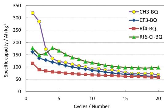
**Fig. 4** Cycle-life performance over twentieth cycles for cells based on CH<sub>3</sub>-BQ, CF<sub>3</sub>-BQ, Rf<sub>4</sub>-BQ, and Rf<sub>6</sub>-Cl-BQ.
