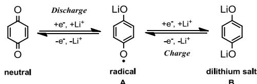
**Scheme 1** Proposed charge-discharge mechanism for benzoquinone as a positive-electrode material in a rechargeable LIB.
