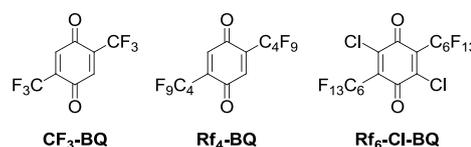
**Fig. 1** Electron-deficient benzoquinones bearing perfluoroalkyl groups.
