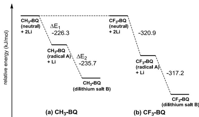
**Fig. 7** Stabilization Energies,  $\Delta E_1$  ( $= (E_{\text{radical}} + E_{\text{Li}}) - (E_{\text{neutral}} + 2E_{\text{Li}})$ ) and  $\Delta E_2$  ( $= E_{\text{dilithium salt}} - (E_{\text{radical}} + E_{\text{Li}})$ ) of (a) CH<sub>3</sub>-BQ and (b) CF<sub>3</sub>-BQ by DFT calculations.
