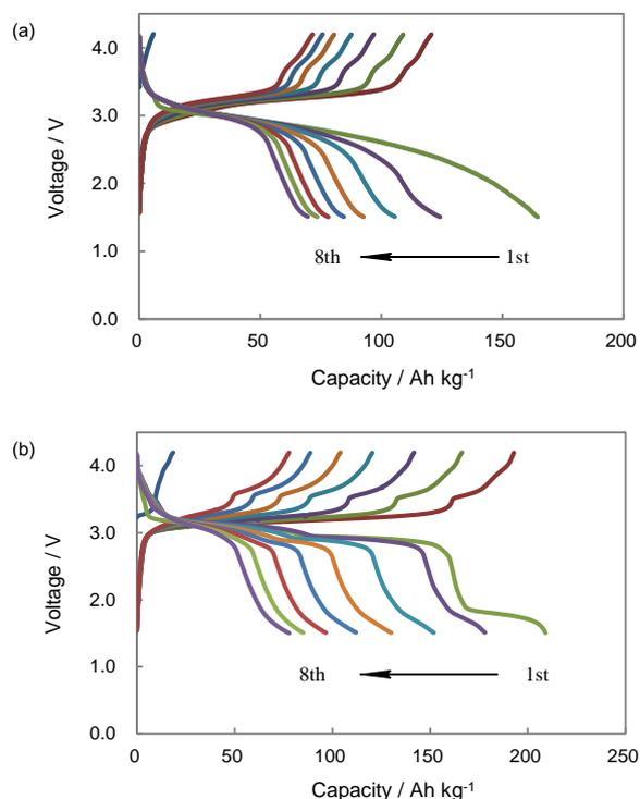
**Fig. 8** Charge-discharge curves and cycle-life performance over eight cycles, using CF<sub>3</sub>-BQ in (a) 4.8 M-LiTFSI in tetraglyme and (b) 1.0 M-LiTFSI in EiPS.
