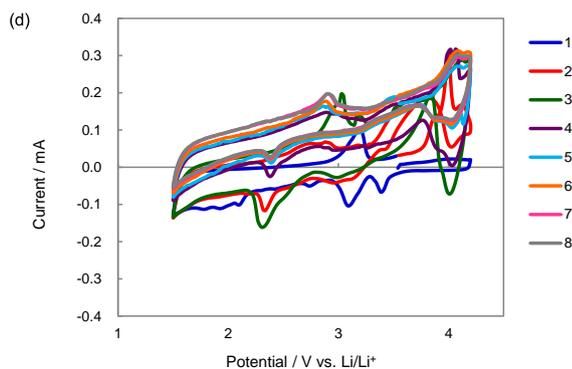
**Fig. 5** Cyclic voltammograms of electrodes containing (a) CH<sub>3</sub>-BQ, (b) CF<sub>3</sub>-BQ, (c) Rf<sub>4</sub>-BQ, and (d) Rf<sub>6</sub>-Cl-BQ in 1.0 M LiPF<sub>6</sub>-EC/DEC. Cycle numbers are indicated by the line colors in the legends
