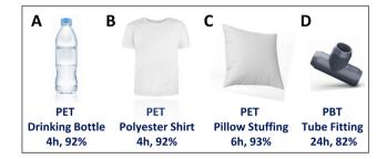
Fig. 4 Aerobic solventless AC/MoO<sub>2</sub>-mediated deconstruction of postconsumer plastic materials A-D. Reaction conditions: 100 mL Schlenk flask, post-consumer polyester stored in air, AC/MoO<sub>2</sub> (3.24 wt% Mo), solventless, 265 °C, air. Yield determined by <sup>1</sup>H NMR using mesitylene internal standard.
