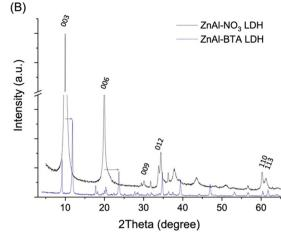
Fig. 3 XRD patterns of (A) Mg-Al LDH-BTA and (B) Zn-Al LDH-BTA.
