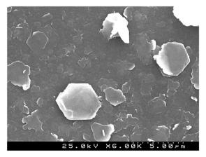
Fig. 2 SEM images of Mg-Al LDH-BTA (left) and Zn-Al LDH-BTA (right)
