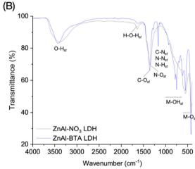
Fig. 4 Fourier transform infrared spectroscopy (FT-IR) spectra of (A) Mg-Al LDH-BTA (A) and (B) Zn-Al LDH-BTA.
