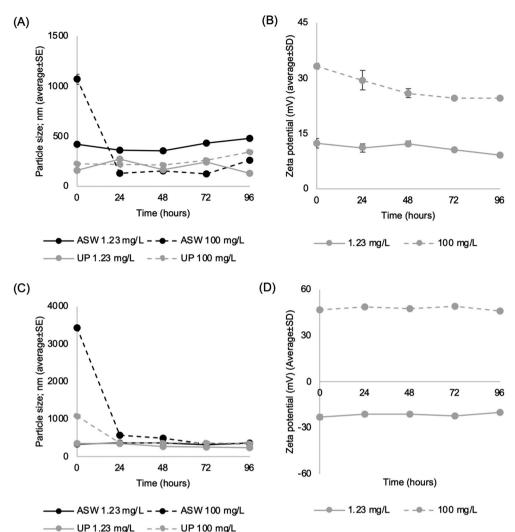
Fig. 7 Effects of concentration and time on the zeta ( $\zeta$ ) potential and particles size of the colloidal dispersions of the anticorrosion nanomaterial Mg–Al LDH–BTA (A and B) and Zn–Al LDH–BTA (C and D) dispersed in ultra-pure water and artificial saltwater, respectively. Dots represent mean values and bars the standard error (SE) for particle size and standard deviation (SD) for zeta potential.
