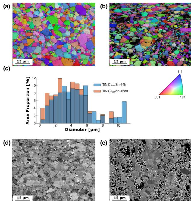
Fig. 3 - Microscopy analysis of  $\text{TiNiCu}_{0.03}\text{Sn}$ . EBSD maps for (a) the 24 h and (b) the 168 h annealed samples; (c) shows the average grain size distribution from the EBSD maps; BSE images of the (d) 24 h and (e) 168 h annealed samples, where greyscale contrast is used to highlight the grains.
