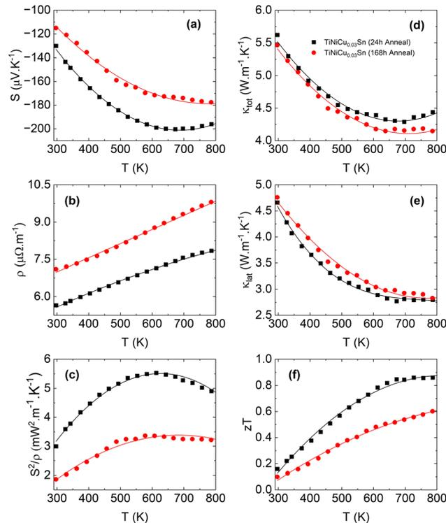
Fig. 2 Temperature dependent thermoelectric properties for the 24 h and 168 h annealed TiNiCu<sub>0.03</sub>Sn samples. Panel (a) shows the Seebeck coefficient  $S$ , (b) the electrical resistivity  $\rho$ , (c) the power factor  $S^2/\rho$ , (d) the total thermal conductivity  $\kappa$ , (e) the lattice thermal conductivity  $\kappa_L$ , and (f) the figure of merit  $zT$ . Lines are guides to the eye.
