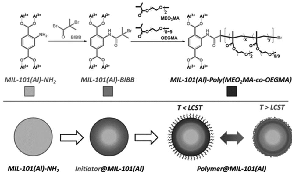
Fig. 3 Synthetic strategy to graft a thermally responsive copolymer from the surface of MIL-101(Al). Schematic illustration at the bottom shows the SI-ATRP process and thermal transition of the grafted polymer. Copyright 2014 Johns Wiley and Sons.
