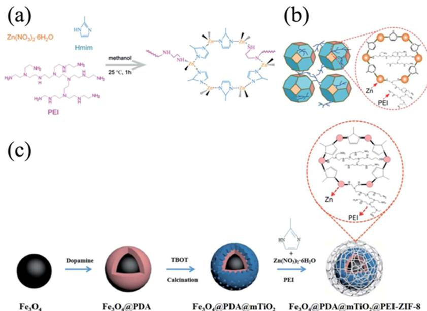
Fig. 12 (a) Synthetic procedure for making PEI-grafted ZIF-8 (b). Copyright 2018 Royal Society of Chemistry. (c) Schematic illustration of the formation of PEI-grafted ZIF-8 onto a functionalized Fe<sub>3</sub>O<sub>4</sub> nanoparticle. Copyright 2020 Royal Society of Chemistry.
