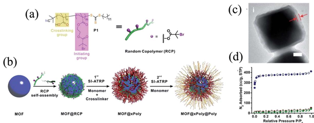
Fig. 7 (a) Chemical formula of the macroinitiator (random copolymer of a carboxylate crosslinking monomer and a bromoisobutyl initiating monomer). (b) Schematic illustration of the SI-ATRP process using a macroinitiator. (c) TEM image of a UiO-66@xPS particle (MOF coated with a crosslinked polystyrene layer); scale bar = 400 nm. (d)  $N_2$  adsorption of pristine UiO-66 (blue), UiO-66@xPS (red), and UiO-66@xPBA (green). Copyright 2019 Royal Society of Chemistry.
