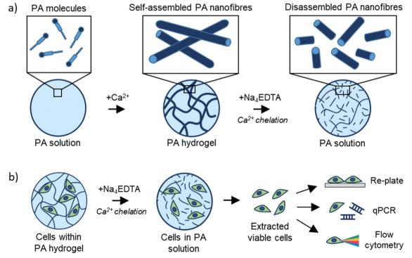
Fig. 1 Rationale of the study. (a) Schematics of PA-E3 molecules self-assembling through CaCl<sub>2</sub> and disassembling through Na<sub>4</sub>EDTA. (b) PA-E3 hydrogels are disassembled to retrieve encapsulated cells for downstream biological analyses.
