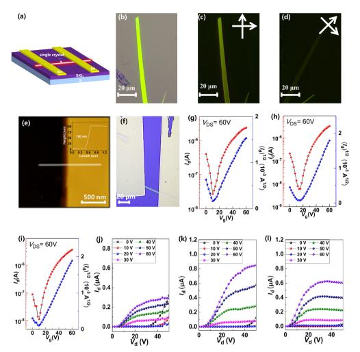
Fig. 9 (a) The device structure of the SC-OFETs; (b-d) OM and POM images of the single crystal of BTPO-I; (e) AFM image of the single crystal of BTPO-I; (f) optical microscopy images of the single crystal of BTPO-I on the SC-OFETs; (q-I) transfer curves and output curves of OFETs based on single crystals of (g and j) BTPO-c, (h and k) BTPO-z, and (i and l) BTPO-l, respectively
