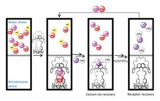
Fig. 27 Schematic illustration of the two-phase extraction through the cation metathesis process by R-85. (Reprinted from ref. 125. Copyright 2012, ACS Publication.)
