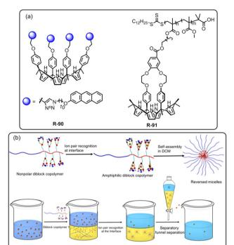
Fig. 25 (a) Chemical structure of the receptors R-90 and R-91. (b) Self-assembly driven micelle formation at the interface by R-91. (Reproduced with permission from ref. 120. Copyright 2018, ACS Publication.)
