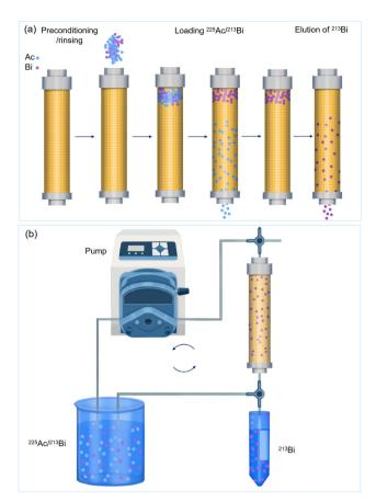
Fig. 11 Simple separation process of the inverse <sup>225</sup>Ac/<sup>213</sup>Bi generator (a) and an automatic separation scheme (b).
