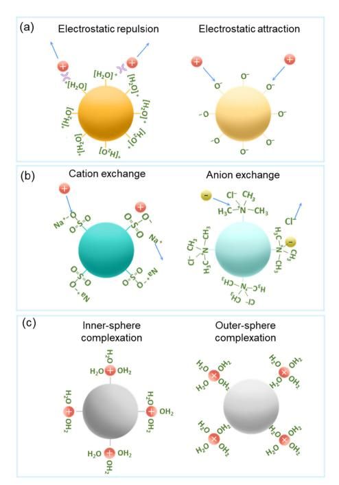
Fig. 7 Schematic diagrams of the adsorption mechanisms: electrostatic interaction (a), ion exchange (b), and surface complexation (c).
