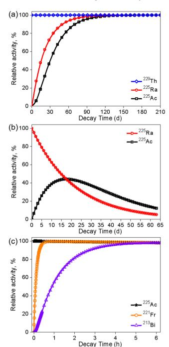
Fig. 6 Theoretical <sup>229</sup>Th-decay and <sup>225</sup>Ra/<sup>225</sup>Ac-ingrowth (a); theoretical <sup>225</sup>Ra-decay and <sup>225</sup>Ac-ingrowth (b); theoretical <sup>225</sup>Ac-decay and <sup>221</sup>Fr/<sup>213</sup>Bi-ingrowth (c).
