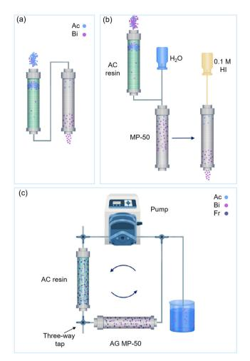
Fig. 10 Separation process of two-column direct <sup>225</sup>Ac/<sup>213</sup>Bi generator, highlighting the functions of second column in further purification (a), both purification and concentration (b), and purification (automatic) (c).
