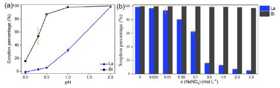
Fig. 17 Sorption percentage of surface-modified activated carbon for La<sup>3+</sup> and Bi<sup>3+</sup> as a function of pH (a) or NaNO<sub>3</sub> concentration (b).<sup>47</sup>
