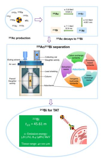
Fig. 2 Schematic diagram of the process from <sup>225</sup>Ac production to <sup>213</sup>Bi for targeted alpha therapy.
