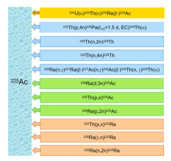
Fig. 3 Nuclear reactions for <sup>225</sup>Ac production.
