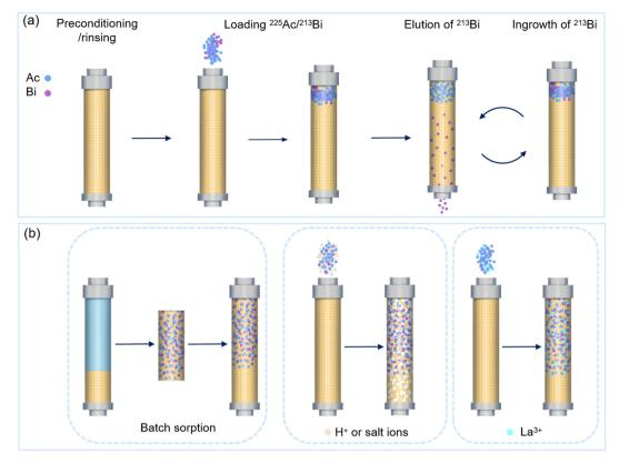
Fig. 9 Separation process of the direct generator system (a) and the loading process to distribute the <sup>225</sup>Ac in a large mass of sorbents (b) (La<sup>3+</sup> acted as a competition ion for Ac3+ sorption).
