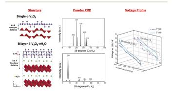
Fig. 7 Structural and electrochemical comparison between crystalline  $V_2O_5$  and bilayered  $\delta$ - $V_2O_5\cdot nH_2O$ . Reproduced and adapted from ref. 23, 102 and 103, with permission from Elsevier, copyright 1994, John Wiley & Sons, copyright 2016, American Chemical Society, copyright 2002.
