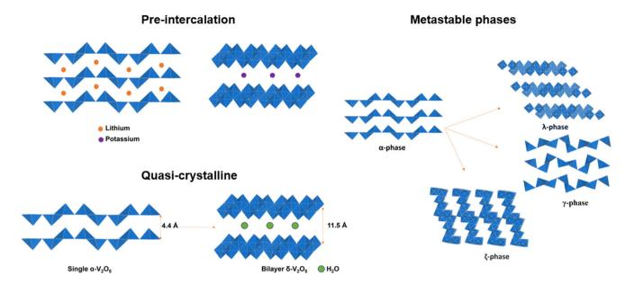
Fig. 2 Structural modification strategies that alleviate distortive phase transformations in  $\alpha$ -V<sub>2</sub>O<sub>5</sub>.
