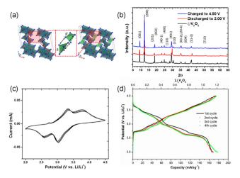
**Fig. 5** Structural and electrochemical data of metastable  $\zeta$ -V<sub>2</sub>O<sub>5</sub>. (a) crystal structures and (b) XRD patterns of  $\zeta$ -V<sub>2</sub>O<sub>5</sub> and lithiated  $\zeta$ -V<sub>2</sub>O<sub>5</sub>. (c) cyclic voltammogram and (d) galvanostatic charge-discharge curves of  $\zeta$ -V<sub>2</sub>O<sub>5</sub>. Reproduced with adaptation from ref. 43 with permission from American Chemical Society. Copyright 2017.
