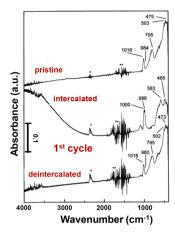
Fig. 9 IR absorption spectra of the  $\rm V_2O_5$  crystalline film at pristine, intercalated, and de-intercalated states. Reproduced with adaption from ref. 129 with permission from Elsevier. Copyright 1999.
