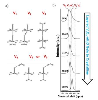
Fig. 12 (a) Different coordination configurations of vanadium sites with water and (b) 51V MAS NMR spectra of V2O5·nH2O gels upon drying. Reproduced with adaption from ref. 34 with permission from American Chemical Society. Copyright 2002.
