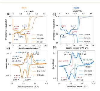
Fig. 3 Charging/discharging profile and cyclic voltammetry data of (a and c)  $\alpha$ -V<sub>2</sub>O<sub>5</sub> microparticle and (b and d)  $\alpha$ -V<sub>2</sub>O<sub>5</sub> nanosphere. Reproduced from ref. 47 with permission from Springer Nature. Copyright 2021.
