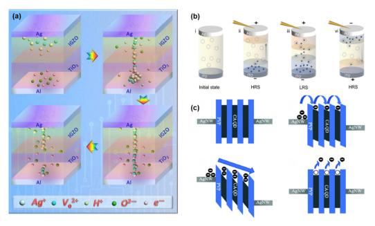
Fig. 4 (a) Schematic illustration of the formation of conductive filaments. <sup>96</sup> (b) Model of the resistive switching mechanism. <sup>118</sup> (c) Schematic band diagrams to explain the resistive switching model. <sup>122</sup> Reprinted with permission from ref. 96, © 2021 American Chemical Society; ref. 118, © 2022 Science China Press and Springer; ref. 122, © 2018 Royal Society of Chemistry.
