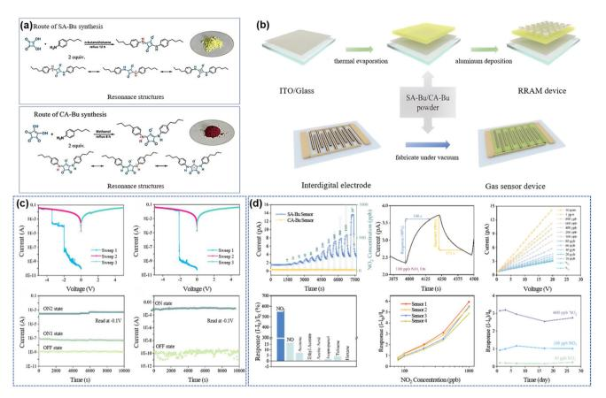
Fig. 6 (a) Synthetic routes of SA-Bu, CA-Bu and their zwitterionic resonance structures. (b) Schematic diagram of fabricating RRAM and gas sensor devices. (c) Typical tri-state I-V and stability test characteristics of SA-Bu/CA-Bu based memory devices. (d) Transient response of SA-Bu and CA-Bu sensors with an increase in NO<sub>2</sub> concentration. <sup>128</sup> Reprinted with permission from ref. 128, © 2021 Elsevier.
