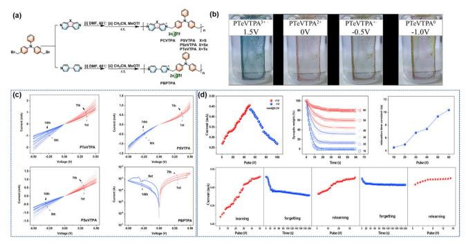
Fig. 7 (a) Synthesis of PCVTPA (PSVTPA, PSeVTPA, PTeVTPA) and PBPTPA. (b) Electrochromic photographs of the PTeVTPA thin film coated onto the ITO substrate. (c) I-V characteristics of the Al/polymer/ITO devices. (d) Synaptic function simulation in human brain memory behavior, including repetitive learning forgetting (STP/STD).<sup>97</sup> Reprinted with permission from ref. 97 © 2021 Open Access.
