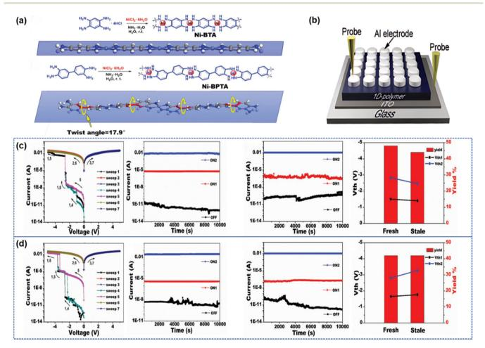
Fig. 8 (a) Synthetic routes and geometry of Ni-BTA and Ni-BPTA. (b) Typical sandwiched structure of memory devices. (c and d) Characteristic I-V curves, stability, threshold voltage and ternary device yield of (c) Ni-BTA and (d) Ni-BPTA.93 Reprinted with permission from ref. 93, © 2017 Wiley.
