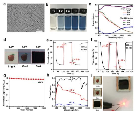
Fig. 5 (a) TEM image and (b) digital photos of TiO<sub>2-x</sub> NCs. (c) Optical transmittance spectra, (d) digital photos, (e and f) switching speed, and (g) cycling stability of TiO<sub>2-x</sub> NC film. (h) Optical transmittance spectra and (i) digital photos of the dual-band EC device. Adapted with permission from ref. 64. Copyright 2020, Wiley-VCH.
