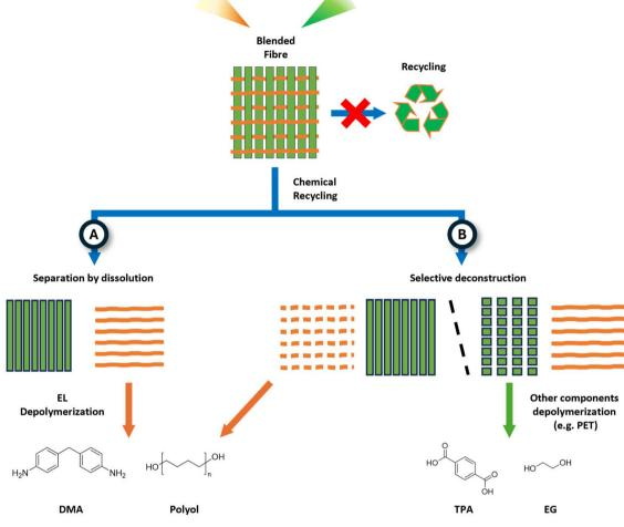
Fig. 14 Schematic of elastane blended fibres and chemical recycling pathways: (A) separation by dissolution and (B) separation by selective deconstruction.
