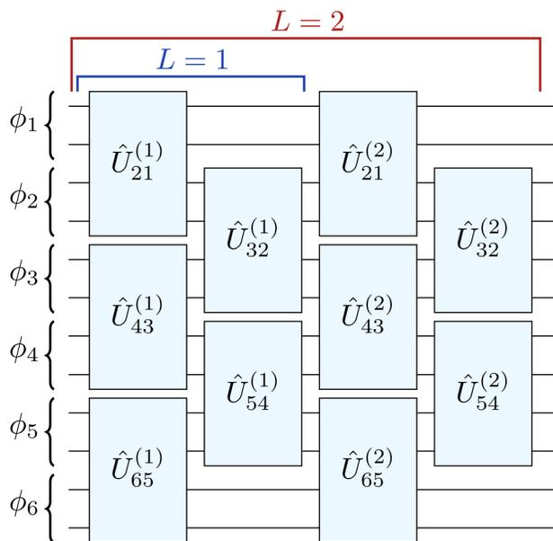
Fig. 1 Circuit structure of the tUPS ansatz.<sup>15</sup> Each qubit encodes the occupation of a spin orbital and the qubits alternate between high- and low-spin orbitals (*e.g.*,  $\phi_1\phi_1\phi_2\phi_2\dots$ ).
