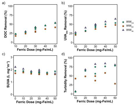
Fig. 2 Percent removals of (a) dissolved organic carbon (DOC), (b) UV<sub>254</sub> absorbance (UVA<sub>254</sub>), (c) specific UV<sub>254</sub> absorbance (SUVA), and (d) turbidity during enhanced coagulation of different secondary effluents.
