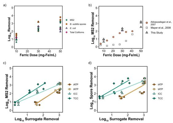
Fig. 4 log<sub>10</sub> removals of spiked microorganisms (a) MS2 bacteriophage, B. subtilis spores, E. coli, and total coliforms with increasing ferric chloride dose; (b) MS2 bacteriophages with increasing ferric chloride doses compared to other bench-scale spiking studies; and (c) MS2 bacteriophage and (d) B. subtilis spore removal with respect to removals of rapid microbial surrogate parameters.
