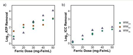
Fig. 3 log<sub>10</sub> removals of (a) total ATP (tATP) and (b) intact cell count (ICC) as determined by flow cytometry, during enhanced coagulation of different secondary effluents. Note: ICC was not measured in Nevada effluent.
