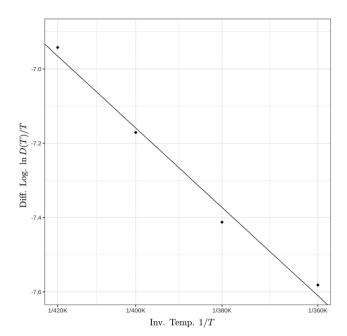
Fig. 8 Natural logarithm of the ratio of the interior diffusion coefficient over temperature as a function of the inverse temperature. The corresponding activation barrier is  $\Delta E^{\ddagger}$  = 3.3  $\pm$  0.3 kcal mol<sup>-1</sup>
