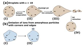
Fig. 10 Schematic of ion emission (a) from droplets of  $\varepsilon > 18$ , and (b) from amorphous particles. The droplet (a) and particle (b) are shown to be charged by negative (-) unbalanced ions because simulations for the N = 4096 GA nano-aggregate have been performed with anions. The same mechanistic steps will also hold for positive ions. Details of the steps are described in the text.
