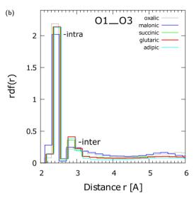
Fig. 1 (a) Numbering of O sites in GA to be used in radial distribution functions (rdf). The same numbering is also followed for all the other diacids examined here. (b) O1-O3 rdf at T = 300 K for various diacids nano-aggregates from OA (C2) to AA (C6) with N=21 molecules
