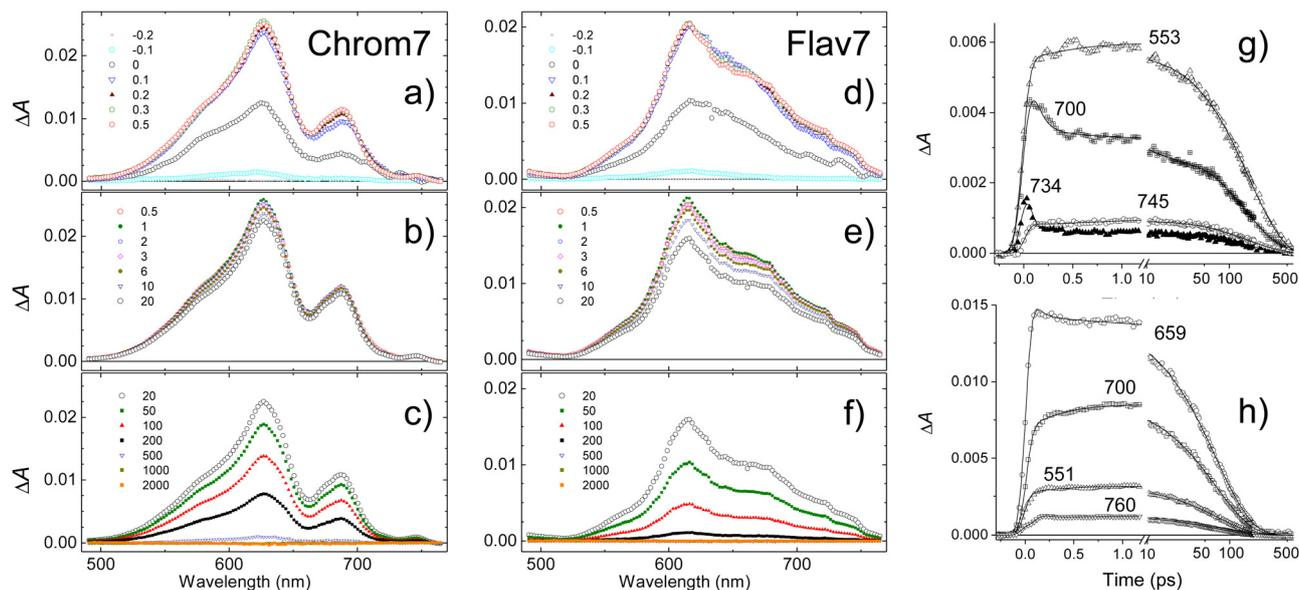
Fig. 4 Transient absorption spectra of Chrom7 (a)–(c) and Flav7 (d)–(f) in  $\text{CH}_2\text{Cl}_2$  at short (a) and (d), intermediate (b) and (e), and long (c) and (f) times following 90-fs 925-nm excitation. Delay times between the excitation and probe pulses are given in the legends. The representative  $\Delta A$  kinetic traces at several probe wavelengths and the fits with CCF deconvolution are shown for Chrom7 in (g) and Flav7 in (h). Note the decadic logarithmic time scale after 10 ps.
