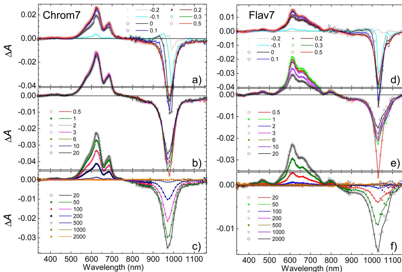
Fig. 2 Short- (a) and (d), intermediate- (b) and (e), and long- (c) and (f) time  $\Delta A$  spectra of 990-nm excited Chrom7 (a)–(c) and 1042-nm excited Flav7 (d)–(f): delay times between excitation and probe pulses expressed in picoseconds are given inside each panel.
