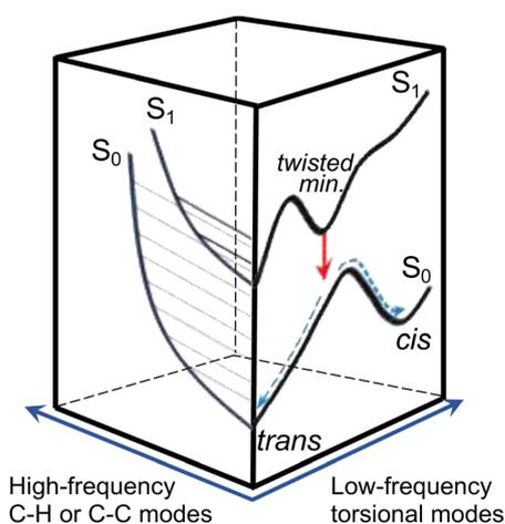
Fig. 9 The radiationless relaxation mechanism of the SWIR polymethine dyes studied in this work with the competing pathways of direct IC, which takes place within the planar  $S_1$  *trans*-form and obeys the energy gap law, and photoisomerization, which is thermally activated. The photoisomerization motion predominantly samples the *trans*-side of the twisted  $S_1$  minimum and is essentially nonreactive.
