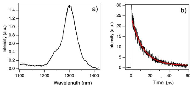
Fig. 7 Phosphorescence spectrum for Chrom7 in a CD<sub>3</sub>I matrix at 77 K, (a) The phosphorescence was recorded in the 4–19 μs time interval after pulsed laser excitation (532 nm, 7-ns pulse width). The phosphorescence decay (black) was measured at a 1300-nm wavelength and can be fitted to a single exponential decay (red) with a 12 μs lifetime, (b).
