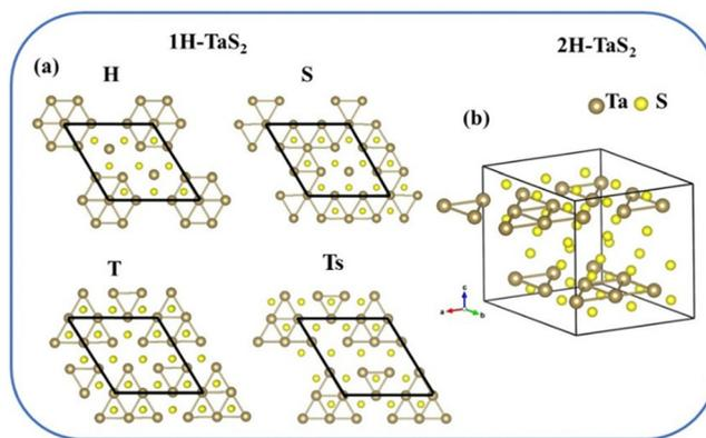
Fig. 1 (a) Four types of possible stable images of CDW phase for mono-layer 1H-TaS<sub>2</sub>. (b) T-Ts configuration of CDW phase for bulk 2H-TaS<sub>2</sub>. Brown spheres represent tantalum atoms while other spheres represent oxygen atoms.
