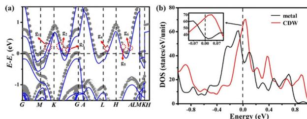
**Fig. 2** (a) Energy band of metal phase and unfolding energy band of CDW phase for bulk sample. The gray and blue lines represent the CDW and metal phases. The  $g_1$ – $g_6$  symbols indicate that the pseudo band gaps are located at the  $g_1$ – $g_6$  points in the BZ, respectively. (b) Total DOS for bulk 2H-TaS<sub>2</sub>.
