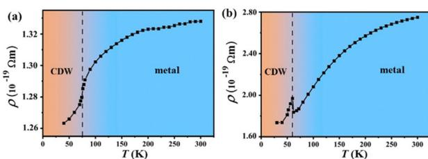
Fig. 4 Temperature dependence of theoretical resistivity for 2H-TaS<sub>2</sub>. (a) Bulk samples, (b) mono-layer samples.
