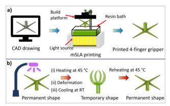
Fig. 1 Schematic presentation of (a) mSLA 3D printing and (b) one-way reversible shape transformation programming controlled by a heat lamp.
