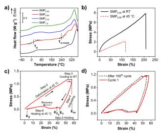
Fig. 3 (a) DSC analysis of 3D-printed SMP<sub>0.33</sub>, SMP<sub>0.50</sub>, SMP<sub>0.75</sub> and SMP<sub>1.0</sub>. (b) Tensile testing of SMP $_{0.50}$  at RT and 45 °C, (c) stress-strain plot for a thermomechanical test cycle, and (d) cyclic thermomechanical test comparison of a specimen of SMP<sub>0.50</sub> after 100 cycles of shape transformation cycle.
