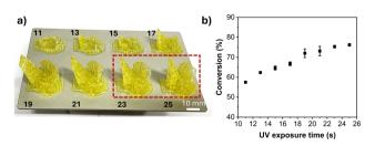
Fig. 2 (a) Printed parts with increasing LED exposure time from 11 to 25 s and (b) corresponding photopolymerization conversion studied by FTIR spectroscopy.
