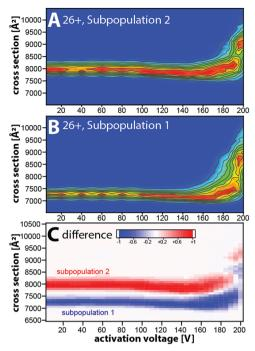
Fig. 3 Conformational heterogeneity of NISTmAb probed by mobilityresolved CIU (mr-CIU) fingerprints obtained via non-ensemble Tandem-TIMS measurements. (A), (B) Mobility-resolved CIU fingerprints of NISTmAb 26+ subpopulations with initial cross-sections centred at  $\sim$ 7260 Å<sup>2</sup> and  $\sim$ 7945 Å<sup>2</sup>, respectively. (C) Difference plot highlighting the differences in the CIU fingerprints of the NISTmAb subpopulations.
