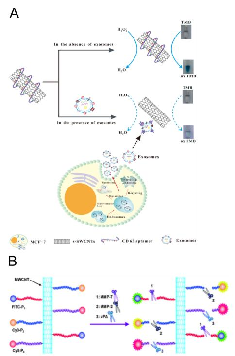
Fig. 8 (A) Principle of the DNA capped single walled carbon nanotube (SWNT)-based aptamer biosensor. Reproduced from ref. 157 with permission from Elsevier, copyright [2017].<sup>157</sup> (B) The principle of the MWCNT-based multicolor fluorescent peptide nanoprobe for the multiplex detection of MMP-7, MMP-2, and uPA. Reproduced from ref. 158 with permission from The Royal Society of Chemistry, copyright [2013]. 158
