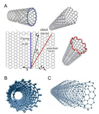
Fig. 2 Different structures of carbon nanotubes in terms of their number of walls. (A) Single-walled carbon nanotube (SWNT) structures according to their chirality (chiral, zigzag and armchair). (B) Model of double-walled carbon nanotubes (DWNTs). (C) Structure of multiwalled carbon nanotubes (MWNTs) consisting of many concentric shells. Reproduced from ref. 33 with permission from Frontiers Media S.A., copyright [2015].33
