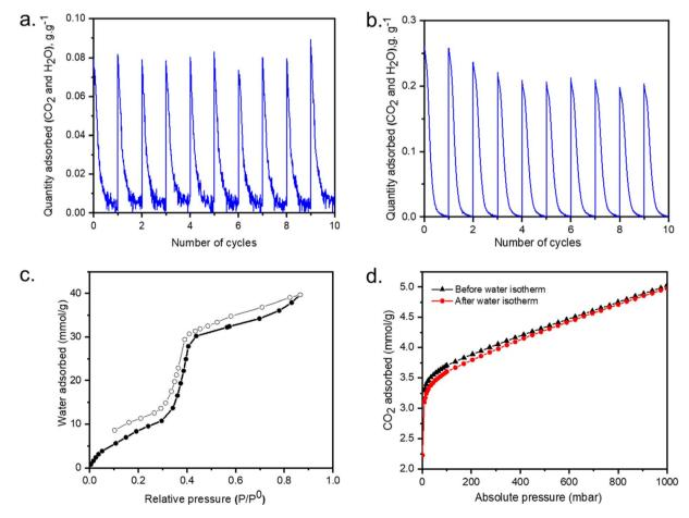
Fig. 5 Regeneration performance cycles at 120 °C for mmen-Mg<sub>2</sub>(dobpdc): (a) after exposing to ambient air with 25% relative humidity; (b) after exposing to ambient air with 45% relative humidity; (c) water isotherm at 25 °C; (d) CO<sub>2</sub> adsorption isotherms before and after measuring water isotherms at 25 °C.
