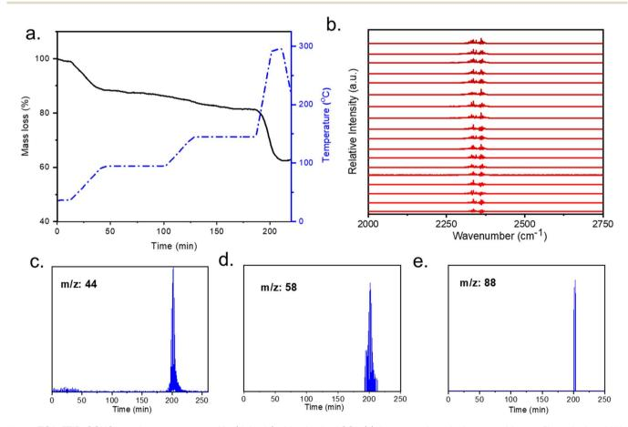
Fig. 4 TGA-FTIR-GCMS experiments on mmen-Mg<sub>2</sub>(dobpdc) with adsorbed CO<sub>2</sub>: (a) thermogravimetric decomposition profile under humid He (black line); temperature ramp rate is shown in blue line; (b) FTIR spectra (0–50 min, 50-100 °C); characteristic CO<sub>2</sub> was detected at 2360 and 2340 cm<sup>-1</sup>, each data was collected every 180 second. (c)–(e) gas chromatography mass spectra (GCMS) showing ions of released amine fragments.
