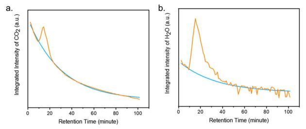
Fig. 7 (a) Integrated intensity of desorbed CO<sub>2</sub> (blue: background, orange: sample) and (b) integrated intensity of desorbed H<sub>2</sub>O (blue: background, orange: sample). Blue curve shows the background intensities of slow displacement of CO2 and H2O from the carrier gas (He), while the orange curve indicates the integrated intensity of the adsorbed CO<sub>2</sub> and H<sub>2</sub>O from the chromatogram.
