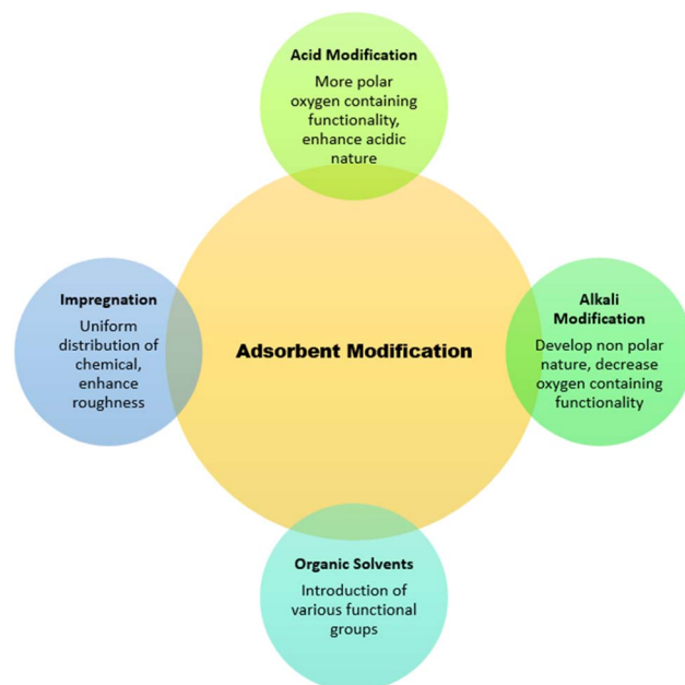
Fig. 4 Types of modification methods of adsorbents and their effects on properties.
