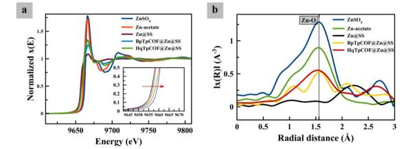
Fig. 3 (a) Zn K-edge XANES spectra at the surface of different zinc electrodes and (b) EXAFS spectra in the R-space for different zinc electrodes at 1 mA h cm<sup>-2</sup> charged in a symmetrical cell.
