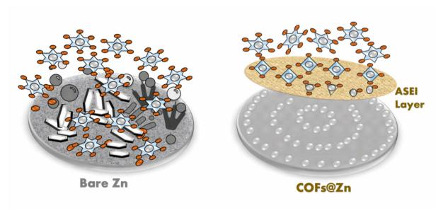
Fig. 8 Scheme illustrates the function of COFs as an ASEI for the Zn anode.
