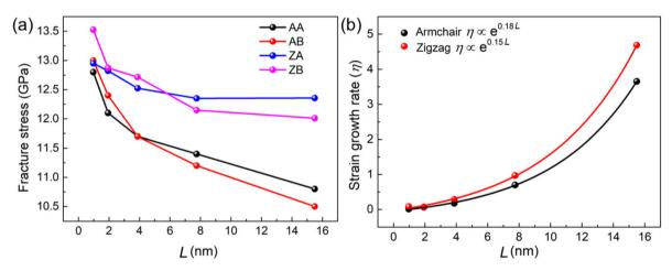
Fig. 6 (a) The obtained fracture of the MoSSe/WSSe heterostructure superlattice versus L; (b) the strain growth rate between the AA (or ZA) and AB (or 7B) at different I
