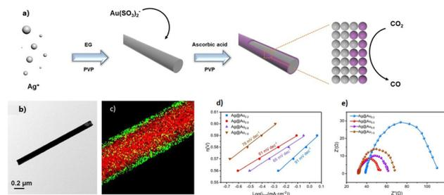
**Fig. 4** (a) Schematic preparation process of Ag@Au core-shell nanowires. (b) Representative TEM image. (c) HAADF-STEM elemental mapping. (d) Tafel slope of Ag@Au<sub>0.2</sub>, Ag@Au<sub>0.5</sub>, Ag@Au<sub>0.8</sub> and Ag@Au<sub>1</sub> electrocatalysts. (e) EIS characterization of Ag@Au<sub>0.2</sub>, Ag@Au<sub>0.5</sub>, Ag@Au<sub>0.8</sub> and Ag@Au<sub>1</sub> electrocatalysts.
