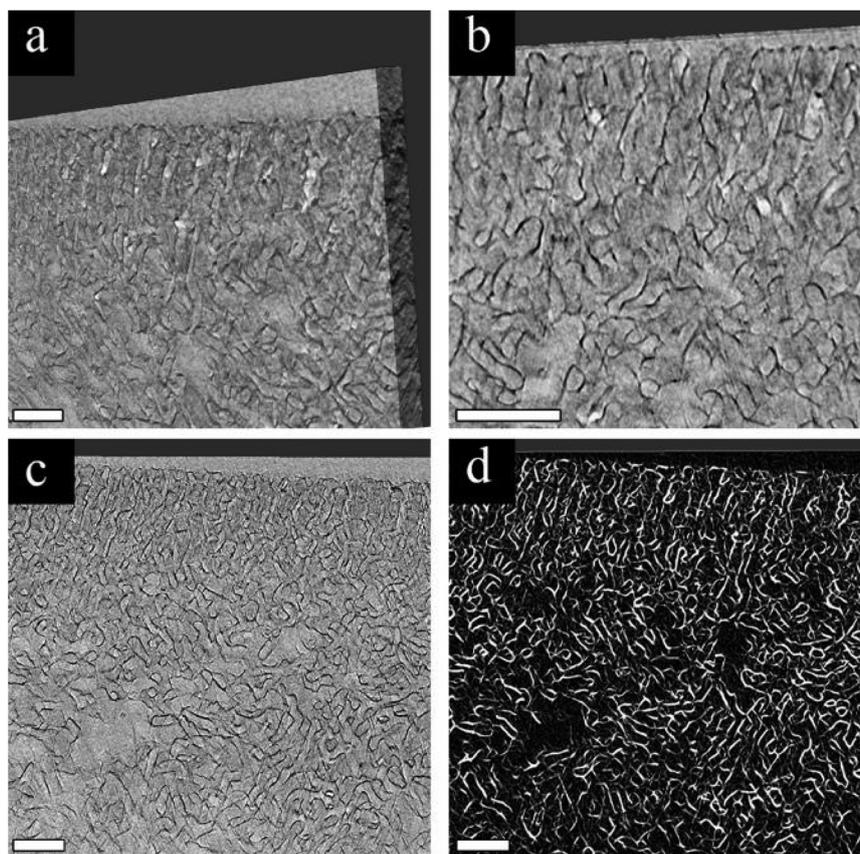
**Fig. 5** TEM tomography of the 25A membrane: (a–b) 3D view of the reconstructed volume at two magnifications, (c) a cross-sectional view from a selected slice, and (d) its segmentation. All the scale bars are 200 nm.
