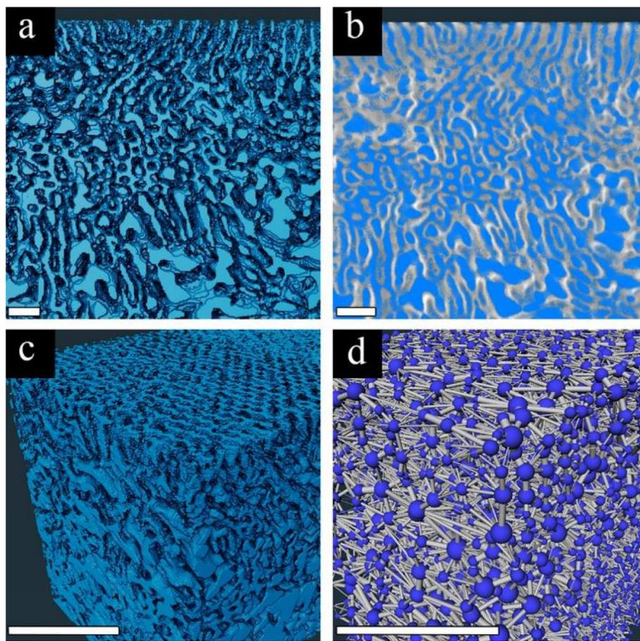
**Fig. 4** Segmentation of the FIB-SEM tomography 3D volume: (a) cross-sectional view of the segmented data, (b) segmentation overlaid with the original data, (c) 3D view of segmented data, and (d) 3D pore network reconstruction performed by using Amira. All the scale bars are 200 nm.
