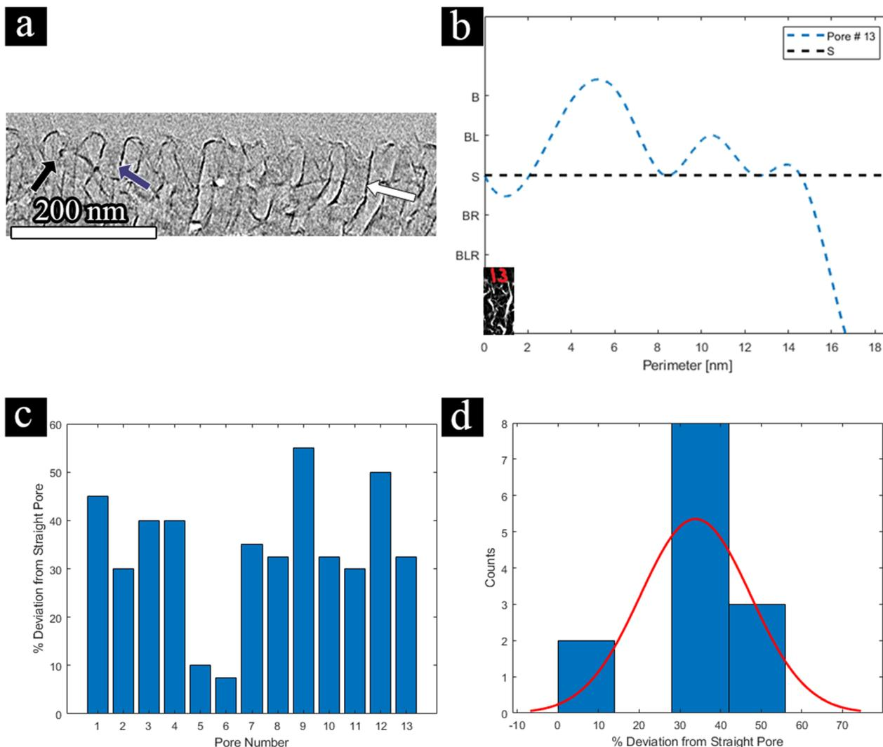
**Fig. 6** TEM tomography analysis – (a) selective slice from the TEM tomography 3D data; the white arrow shows a Double-Wall Curved Bend pore (B), the black arrow shows a Single-Wall Bend left pore (BL), and the blue arrow shows a Straight pore (S), (b) a perimeter profile of a single pore #13 at  $p=0$  nm (inset), (c) deviation from a straight pore for 13 selected pores, (d) a histogram of the deviation from a straight pore.
