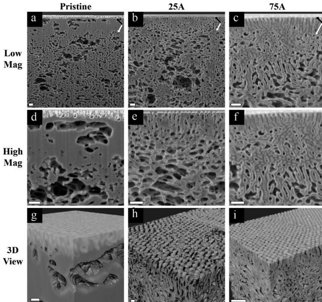
**Fig. 3** (a–f) Cross-sectional SEM images and (g–i) reconstructed 3D volume of pristine membrane (a, d and g) and membrane modified with 3 cycles of  $\text{AlO}_x$  SIS and 25 (b, e and h) or 75 cycles of  $\text{AlO}_x$  ALD (c, f and i). Images d–f are higher magnifications of images a–c, respectively. The black arrows point to the highly ordered selective layer and the white arrows to the underneath supporting layer. All the scale bars are 200 nm.
