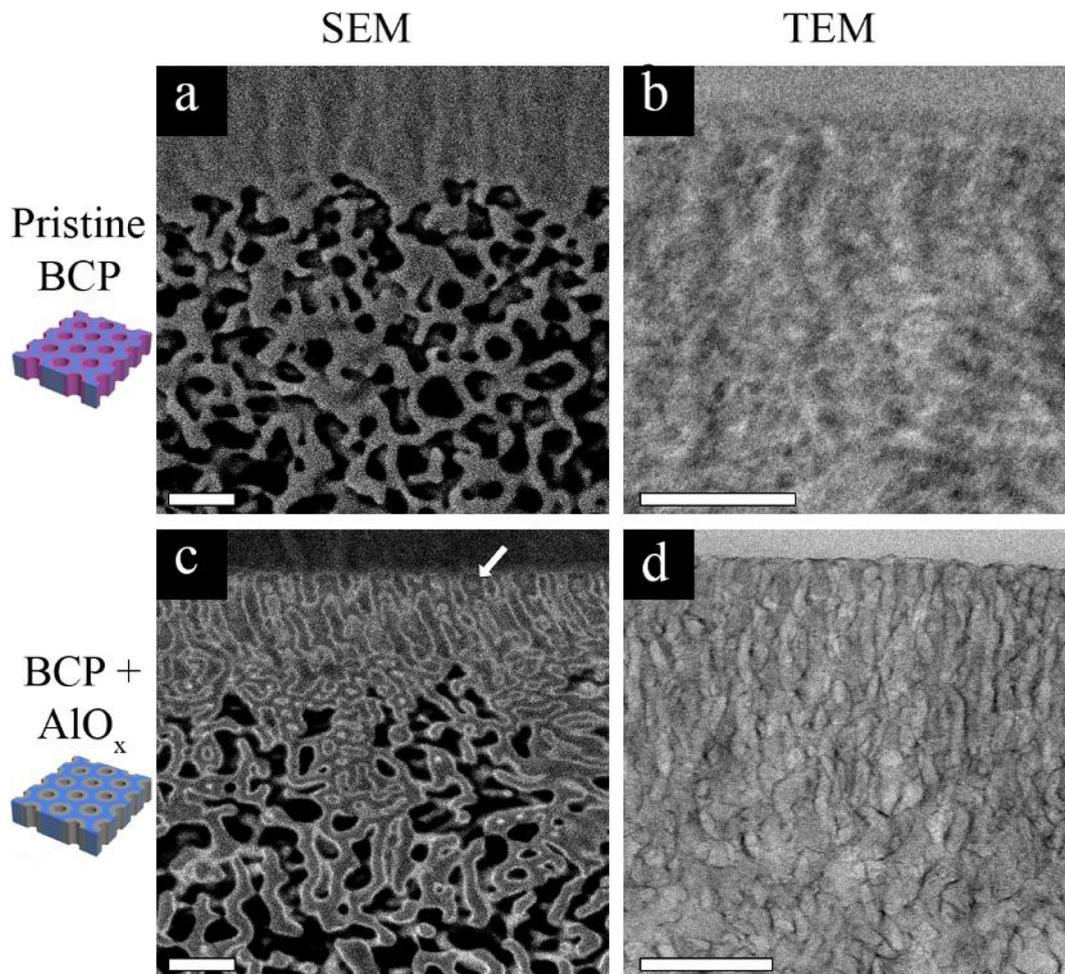
**Fig. 1** Cross-sectional EM images. (a) BSE-SEM of a pristine membrane and (b) its corresponding TEM (b); (c) BSE-SEM of a membrane modified with  $\text{AlO}_x$  by SIS and ALD (the white arrow point to the top surface) and (d) its corresponding TEM. All the scale bars are 200 nm.
