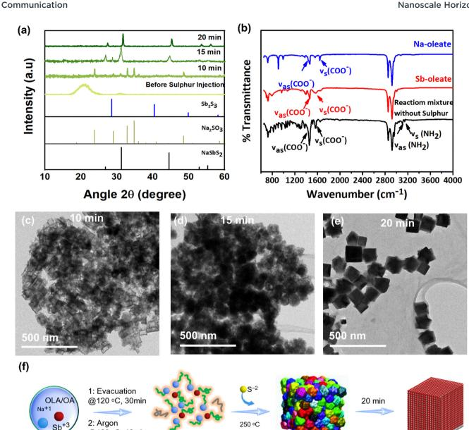
Fig. 5 (a) XRD spectra showing the phase evolution of NaSbS<sub>2</sub> NCs at different reaction time i.e. before injection of sulphur and after injection of sulphur precursor (10, 15 and 20 min) along with (b) FTIR spectra of aliquot taken before injection of sulphur. Panels (c and e) show the TEM images for 10, 15 and 20 min respectively. (f) Schematic depiction of time lapsed phase evolution of NCs.
