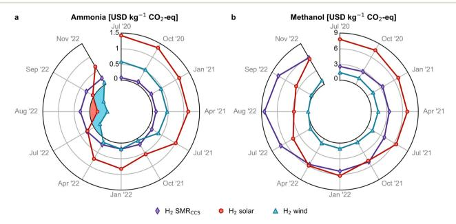
Fig. 4 Avoidance costs for green (a) ammonia and (b) methanol production routes. A negative avoidance cost (blue and red shaded region) implies that it is possible to reduce costs and greenhouse gas (GHG) emissions simultaneously. Monthly analyses with error bars are available in Fig. S17.†
