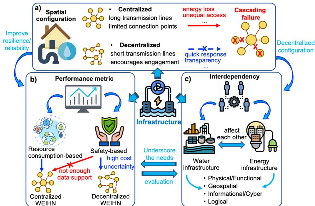
Fig. 3 The comprehensive scheme of the roles of infrastructure in WEIHN. a) The spatial configuration performance in the centralized and decentralized WEIHN. b) The performance metric in the centralized and decentralized WEIHN. c) The interdependency between water and energy infrastructures.
