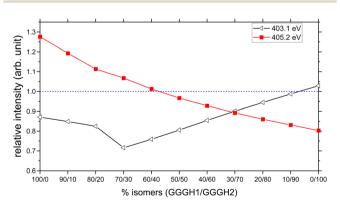
Fig. 7 Relative intensities of the calculated resonances at 403.1 eV (black,  $\sigma^*$ (NH) of the unprotonated – NH<sub>2</sub> group) and at 405.2 eV (red,  $\sigma^*$ (CH) from the backbone), compared to the experimental ones, as a function of the isomer mixing ratio GGGH1 and GGGH2. The dashed blue line represents a relative intensity of 1.
