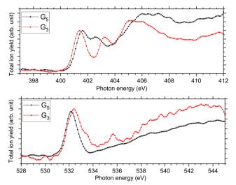
Fig. 4 Experimental NEXAMS spectra at the N K-edge (top) and at the O K-edge (bottom) of G<sub>5</sub> in black and G<sub>3</sub> in red.
