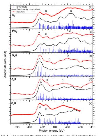
Fig. 3 The experimental nitrogen K-edge total ion yield spectra for G<sub>5</sub>,  $PG_4$ ,  $G_4H$ ,  $G_4R$ , and  $G_4K$ , are shown with red dotted lines. In blue, the DFT/ ROCIS X-ray absorption lines are displayed for each molecule. The absorption lines were shifted by  $\sim 13$  eV and were broadened using a Pseudo-Voigt profile with a 0.6 eV FWHM represented in black.
